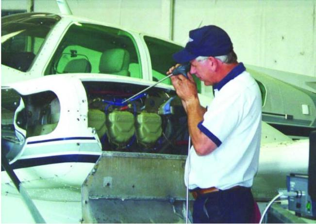
Inspect each cylinder for signatures of normal wear (Figure 4). Cylinder walls which appear to have minimal, or no hone pattern are acceptable if the cylinder has acceptable differential compression readings and the engine has acceptable oil consumption.
